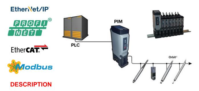
Solartron Metrology's Protocol Interface Module (PIM) provides a simple way of interfacing the Orbit® Digital Measuring Network to most Programmable Logic Controllers (PLCs). A distinct PIM is created for each protocol, including:
